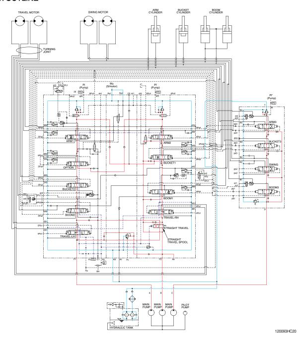
The oil from the A, B and C pump flows through the neutral oil passage, bypass oil passage and confluence oil passage in the main control valve. Then the oil goes to each actuator and operates them. Check valves and orifices are located on these oil passage in the main control valve. These control the oil from the main pumps so as to correspond to the operation of each actuator and smooth the combined operation.
