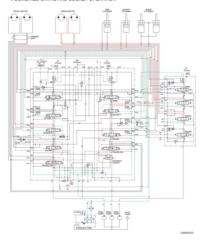
When the swing and bucket functions are operated, simultaneously the swing spool and bucket spools in the main control valve are moved to the functional position by the pilot oil pressure from the remote control valve.
