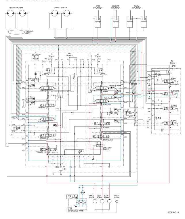
When the RH control lever is pulled left, the bucket spools in the main control valve are moved to the roll in position by the pilot oil pressure from the remote control valve.
