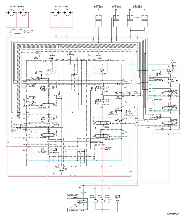
When the swing and travel functions are operated, simultaneously the swing spool and travel spools in the main control valve are moved to the functional position by the pilot oil pressure from the remote control valve and straight travel spool remained its position because the pilot oil pressure from the pilot pump is not applied to the straight travel spool.
