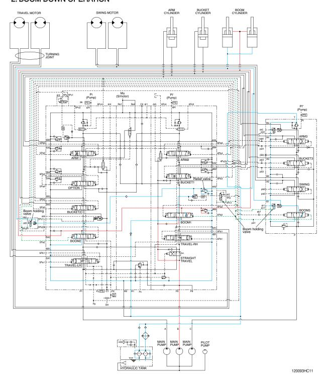
When the RH control lever is pushed forward, the boom 1 spools in the main control valve are moved to the down position by the pilot oil pressure from the remote control valve.
