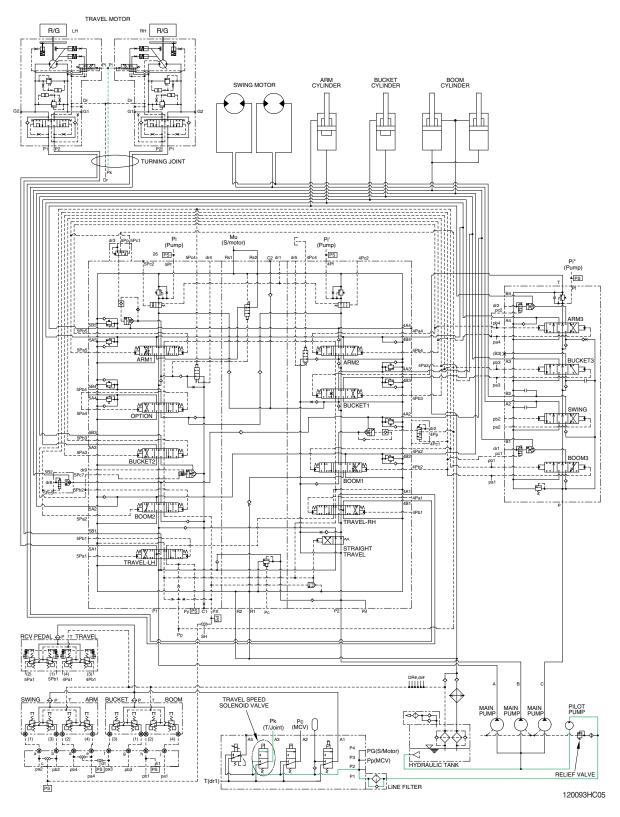
When the travel speed control switch is selected to the high speed, the travel speed solenoid valve is actuated and the discharged oil from the pilot pump flows to the **Pi** port of pilot valve in the travel motors.
