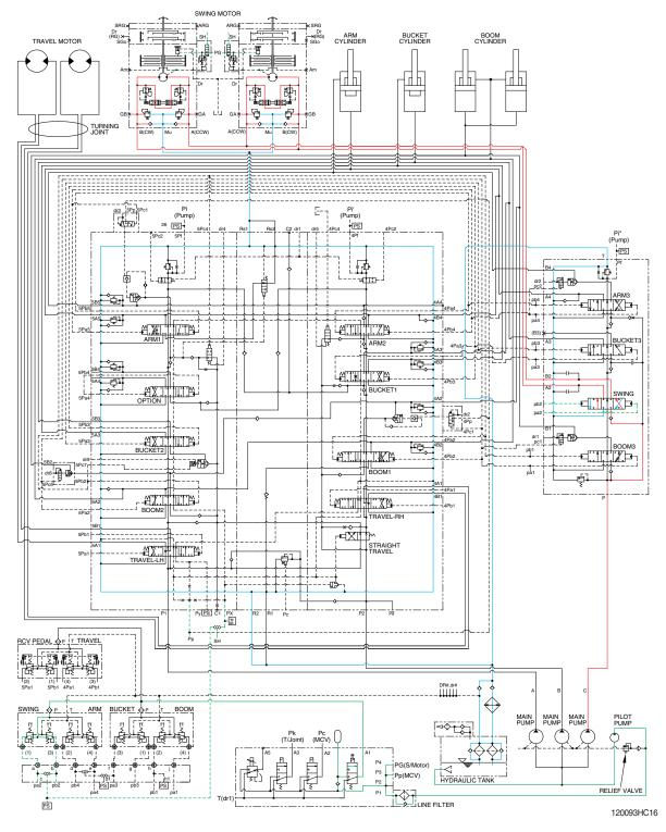
When the LH control lever is pushed left or right, the swing spool in the main control valve 2 is moved to the left or right swing position by the pilot oil pressure from the remote control valve.
