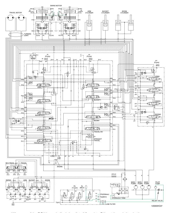
When one of the RCV levers is tilted, the pilot oil flows into SH port through the shuttle.
