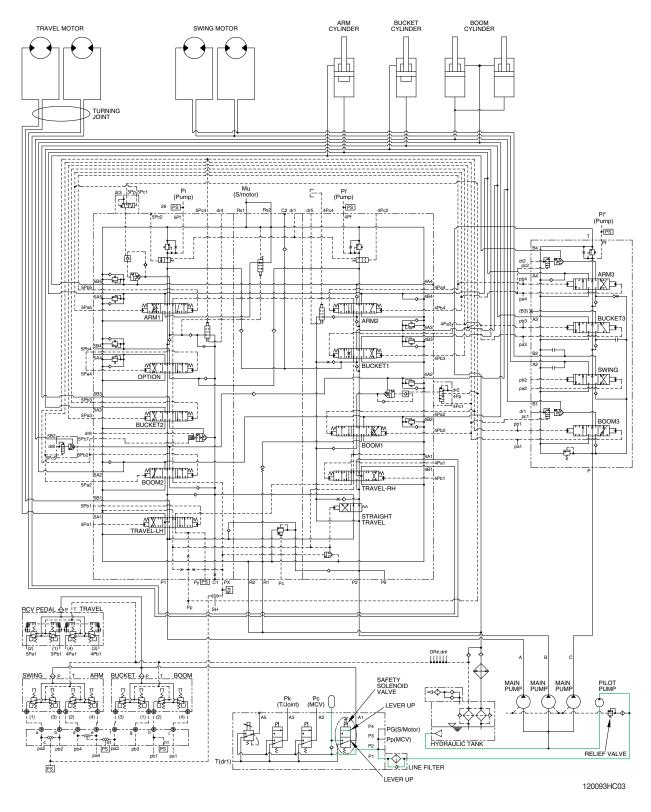
When the lever of the safety solenoid valve is moved downward, oil flows into the remote control valve through solenoid valve and line filter.
