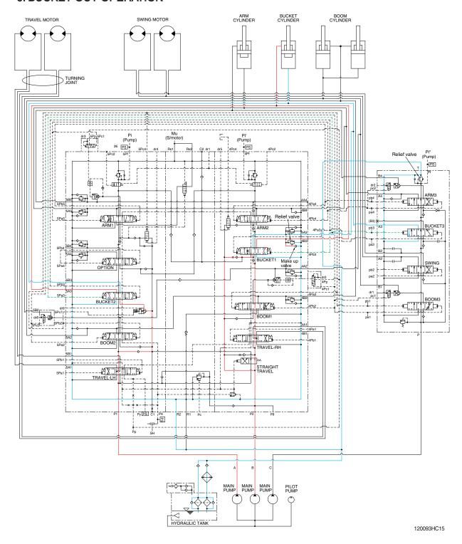
When the RH control lever is pushed right, the bucket spools in the main control valves are moved to the roll out position by the pilot oil pressure from the remote control valve.
